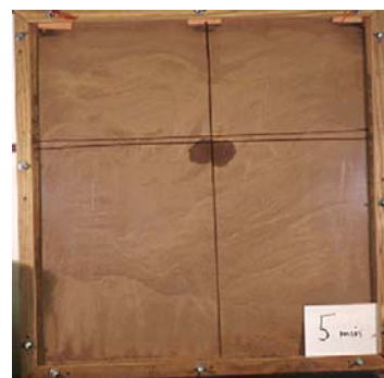
A single emitter (rate 0.61 gph) is placed in dry soil. Note the pattern of the wetting front.
