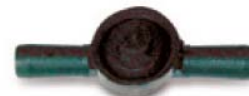
TLCV Inline Check Valve • Flow Range: 0.9 to 4.4 GPM • Opening Pressure: 7.1 psi • Closing Pressure: 5.7 psi
