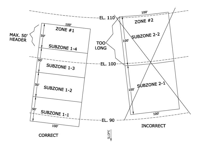
"Top Feed Manifolds" should be utilized on all sites with discernable slope. When using "Top Feed Manifolds", zones should be broken into subzones with no subzone header being longer than 50'. The above schematics show zone #1 correctly being broken into multiple zubzones with headers no longer than 50'. The schematic also shows zone #2 incorrectly being broken into subzones with 100' header.
